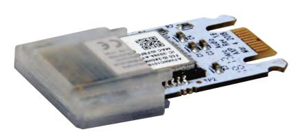
Once installed, the AXP requires use of either a Mobile Hot Spot or a Wi-Fi router connection to connect the two devices together. After initial setup and connection, the system will easily re-connect like a default (preferred) connection point.
